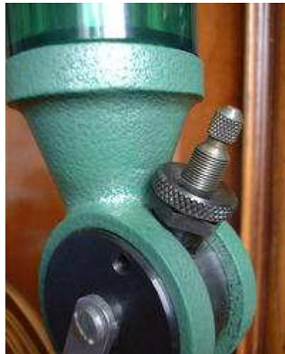
Photo N°2 DOSEUSE VOLUMETRIQUE
